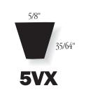
Combine cross section designation with Outside Circumference (O.C.) to the nearest whole number, plus a zero to determine Belt Part Number. Example: 5/8" top width 5VX belt with 80" O.C. equals 5VX800 V-Belt. X designates molded notch construction.
