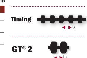
**Example:** TP1200-8MGT-20 Belt (GT2) Twin Power® PowerGrip® GT® 2 Belts Stock Belt Pitch Reference Dimension A 3mm 3mm .118 in. 5mm 5mm .197 in. 8mm 8mm .315 in. 14mm 14mm .552 in. 3, 5, 8 & 14mm PowerGrip GT2 available in the standard single sided belt widths
